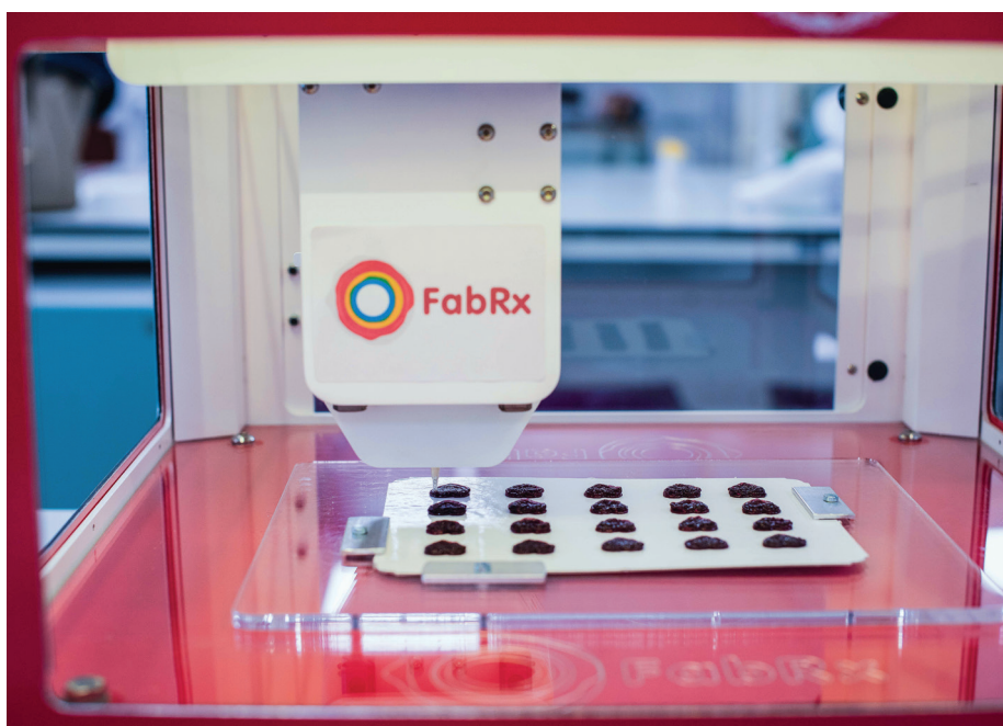
Figure 3: FabRx's semi-solid extrusion 3D-printing process to create chewable printlets – ideal for treating children.
