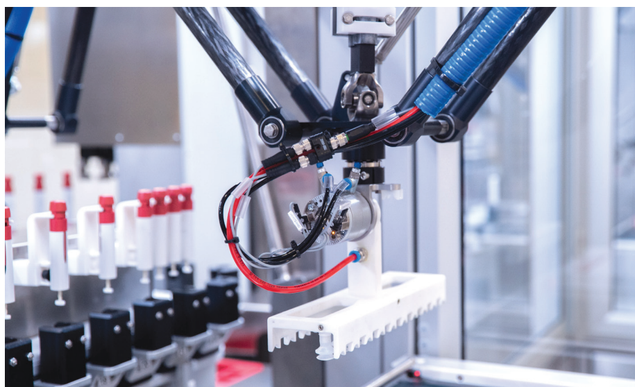
Figure 4: Flexible and modular assembly line developed and produced at Stevanato Group for pen injectors.
