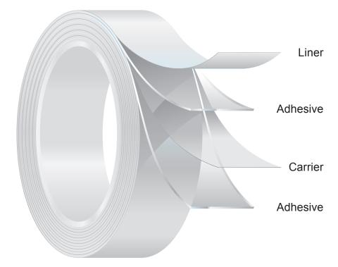
Figure 1: The construction of a double-coated PSA medical tape. This type of tape is commonly used in wearable medical devices.
