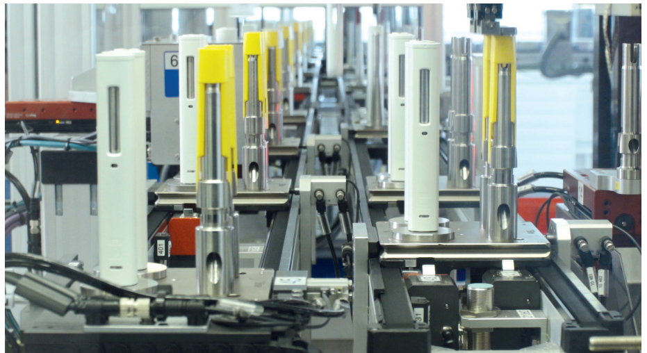
Figure 3: Fully automated assembly with validated process and IPC for YpsoMate and YpsoMate 2.25 (YpsoMate 2.25 pictured).
