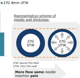
Injection forces simulated using a mathematical model for injections. The model relies on Bernouilli and Poiseuille equations for fluid and pressure drop simulation respectively. Values represented were obtained with assumptions relative to manual SC injection for three needle configurations and fluid viscosities.<sup>15</sup>
