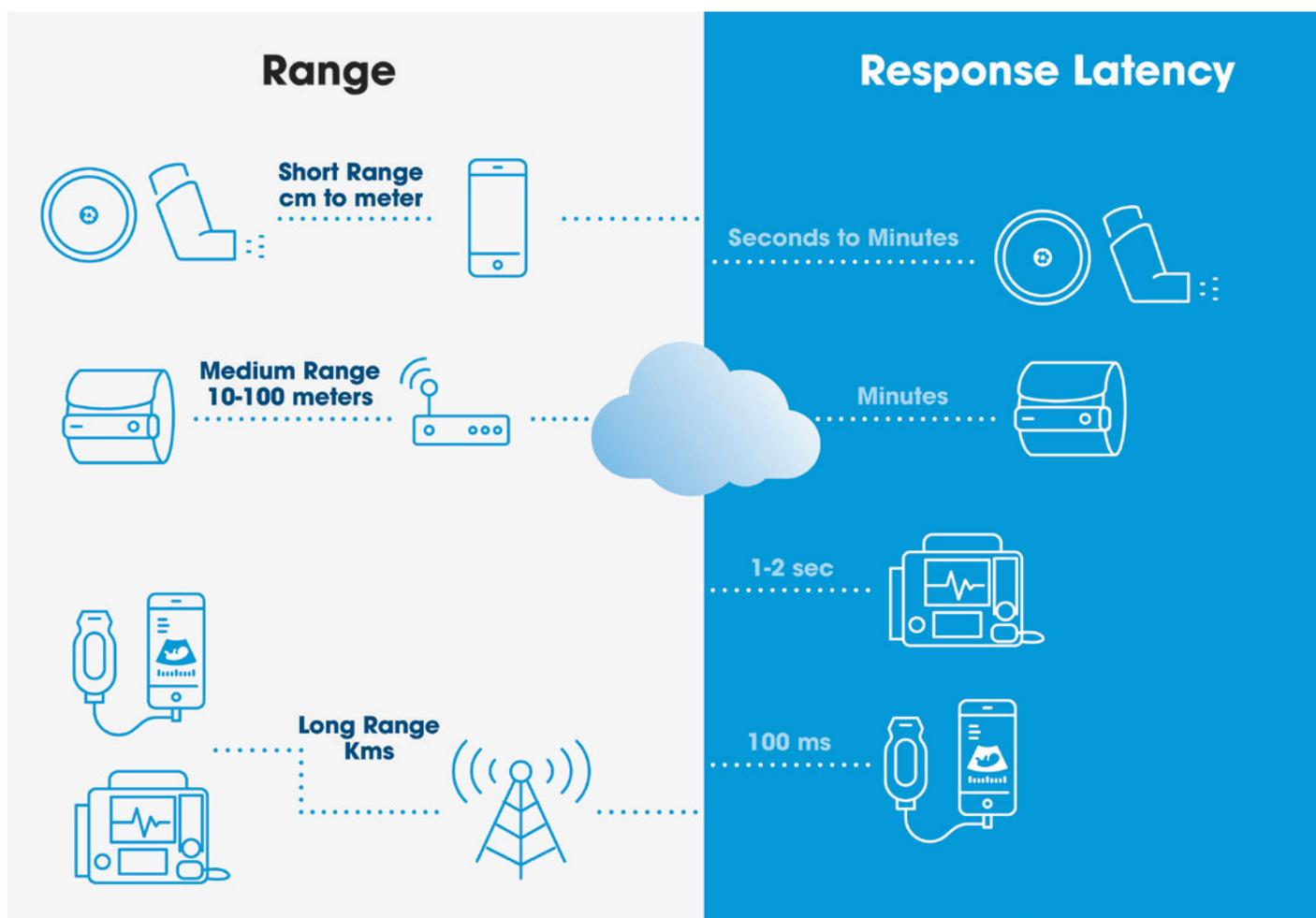
Figure 1: Example of device classifications based on range and latency.
