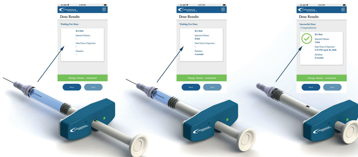
Figure 3: Automatic data capture, real-time feedback and dose history.
