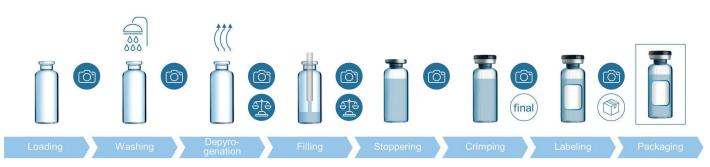
Figure 3: Laser-marked containers and cameras located at different positions on the filling line allow each individual item to be tracked throughout the fill-and-finish process.
