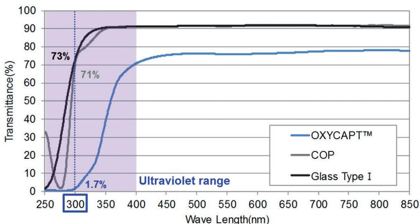
Figure 4: UV light transmittance comparison of a typical COP, Type I glass and OXYCAPT™.
