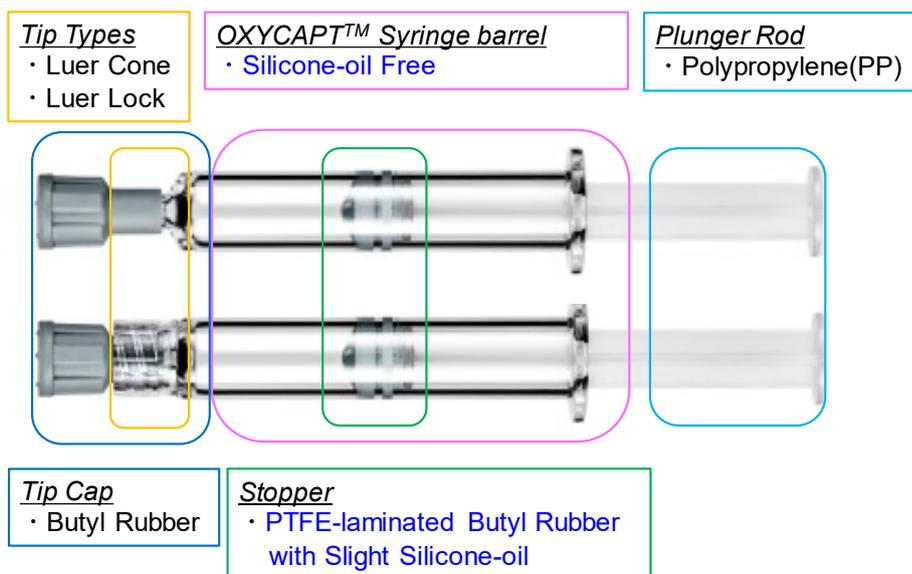
Figure 6: Components of an OXYCAPT™ syringe.
