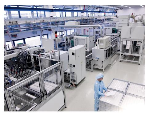
Figure 2: Stevanato Group has more than 160 injection moulding machines at three locations in the US and Germany for GMP, ISO 8 and ISO 7 cleanroom production.
