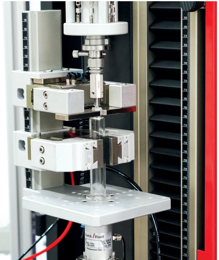
Figure 1: Luer lock testing in accordance with ISO 80369, as performed on a zwickiLine testing machine with testXpert testing software. The zwickiLine fulfills the requirements set out by the US FDA in 21 CFR Part 11.
