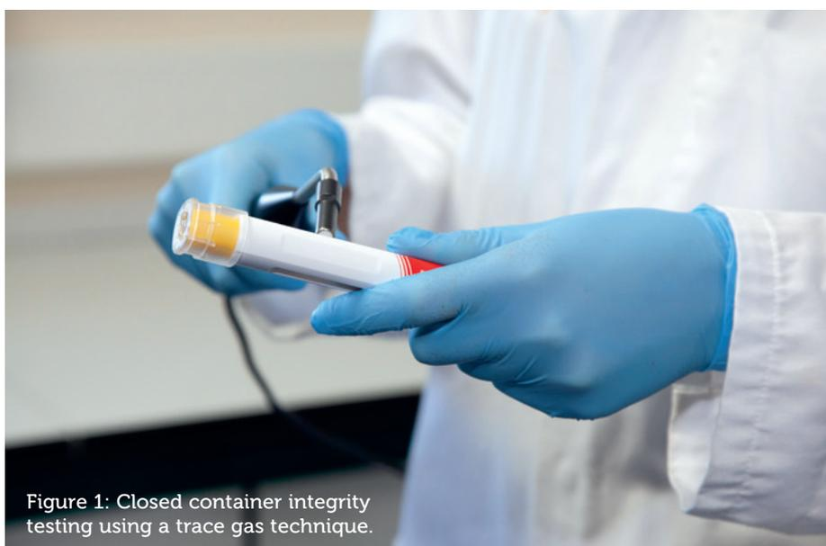
Figure 1: Closed container integrity testing using a trace gas technique.
