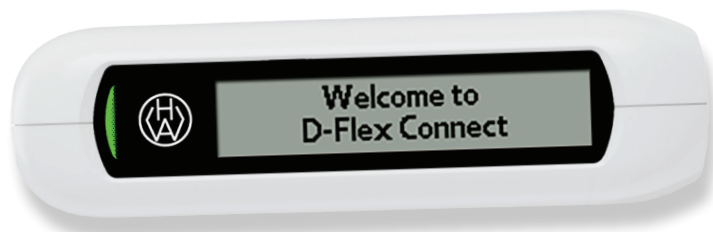
Figure 3: The D-Flex® Connect cap works seamlessly with the D-Flex® injection pen to provide easy data collection and transfer, and facilitates analysis of data sets and dosage adjustments.
