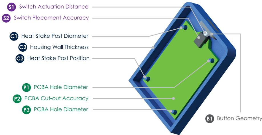
Figure 2: Factors contributing to button actuation profile accuracy.
