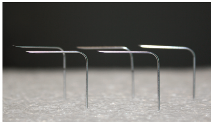
Figure 3: To ensure 100% safe use and functionality of the medical device, precise and repeatable needle bending needs to accommodate the input of imprecise bulk needles.
