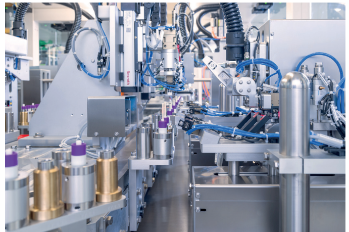
Figure 2: teamtechnik's high-speed assembly solution for pen injectors.
