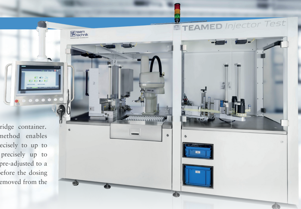
Figure 5: The offline TEAMED test bench is a testing system for batch approval and quality assurance.
