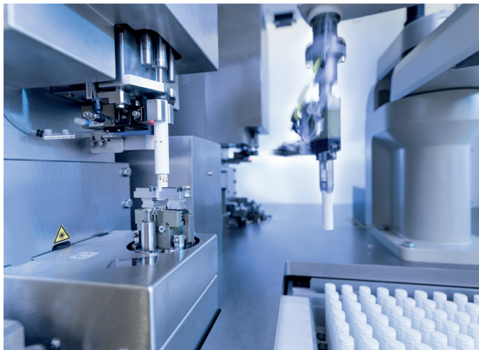
Figure 6: teamtechnik achieves dynamic torque and force testing in a single process.
