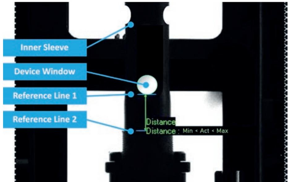
Figure 3: With 100% in-line controls, sensors can check, amongst other things, if device components are in the correct position, and if not, automatically reject the device.
