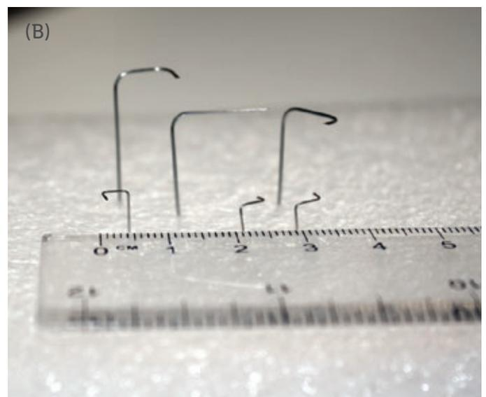
Figure 4: Complex geometries (A) and thinner and smaller cannulas (B) mean that needle handling is challenging and demands expertise for the design of the process station.
