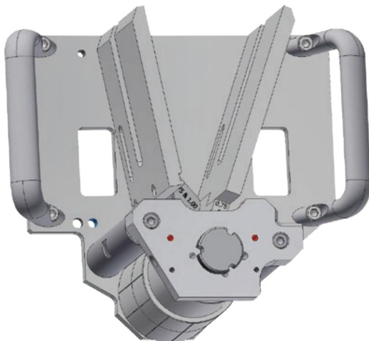
Figure 1: An example of a cannulator with V-shaped hopper for singulation of bulk needles.
