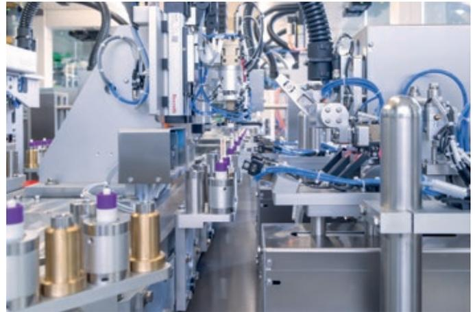
Figure 2: teamtechnik's high-speed assembly solution for pen injectors.
