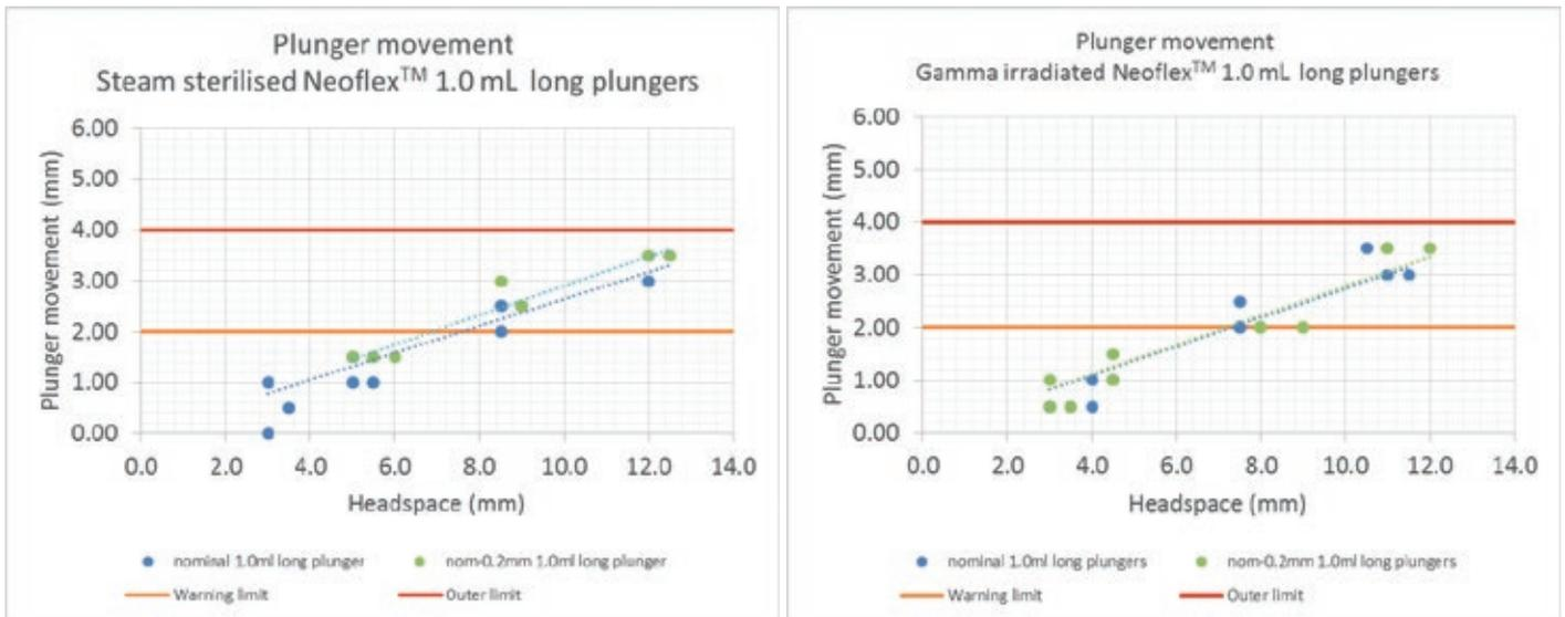
Figure 3: The above graphs show that, for plungers in a highly pressurised setting, plunger movement is minimal and well below the outer limit, regardless of whether the plungers were steam sterilised or gamma irradiated.
