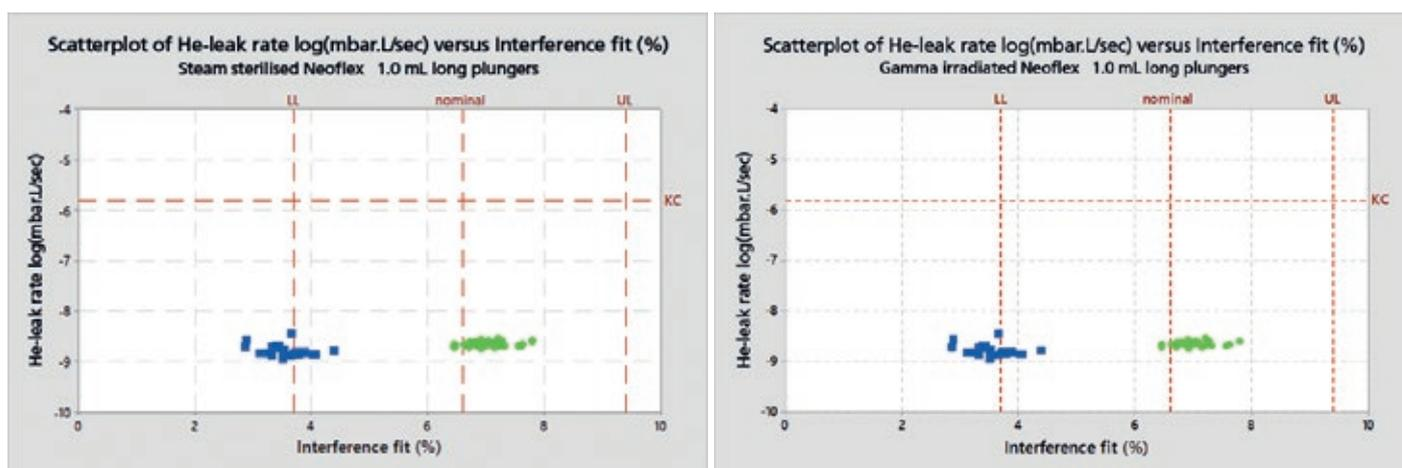
Figure 1: He-leak rates of gamma irradiated 1 mL long NeoFlex plungers with different interference fits. All cases easily meet the Kirsch Criterion ( $1.6 \times 10^{-6}$  mbar.L/sec). Even with the worst-case scenario of a low interference fit, the seal integrity is still maintained.
