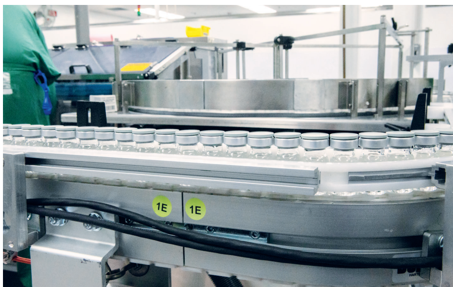
Figure 2: A vial fill line usually uses in-house processed glass before the vial enters the aseptic fill suite.
