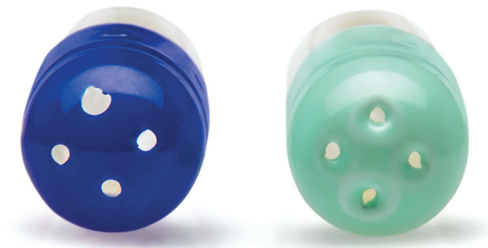
Figure 6: Gelatin capsules with uneven punctures. HPMC capsules with even punctures and no fragmentation.
