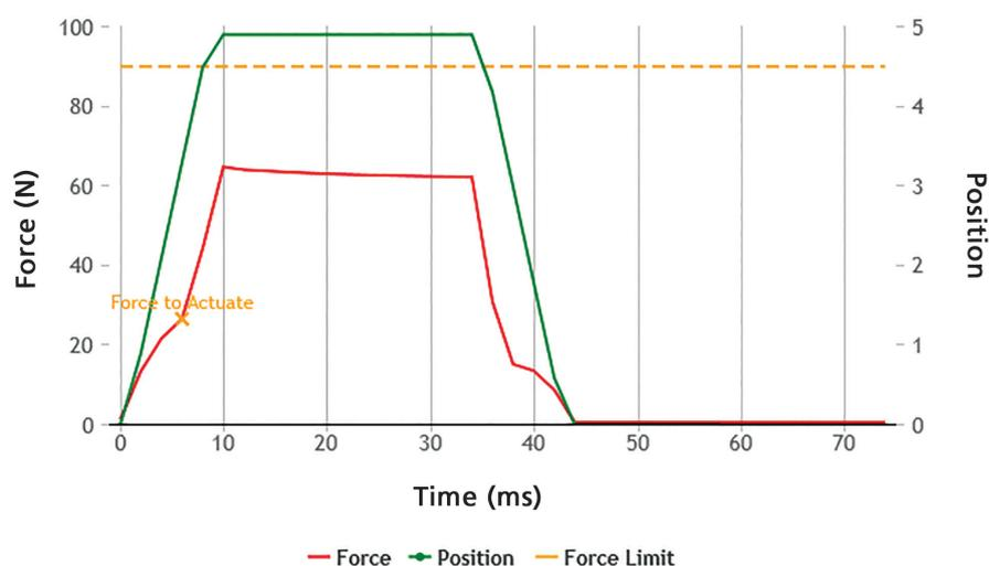
Figure 2: Proveris instrument users can create and evaluate products using force/position versus time plots generated by the system software.
