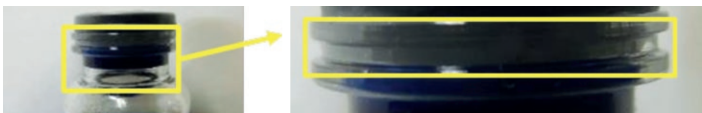
Figure 9: Examination of OXYCAPT vial after storage at -180°C.
