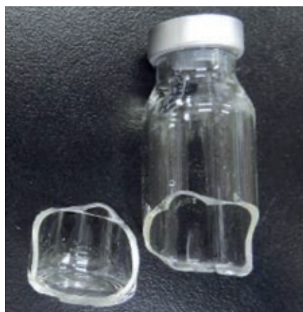
Figure 7: Broken COP vial after drop test following storage at -180°C.
