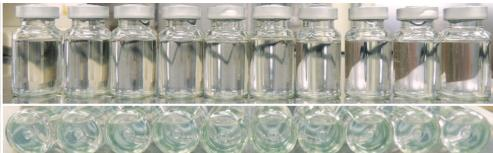
Figure 6: No breakage, leakage or layer separation was found after the quick defrosting test (-80°C to 40°C).
