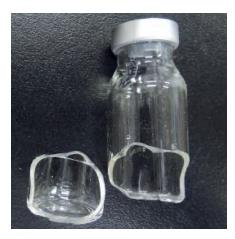
Figure 7: Broken COP vial after drop test following storage at -180°C.
