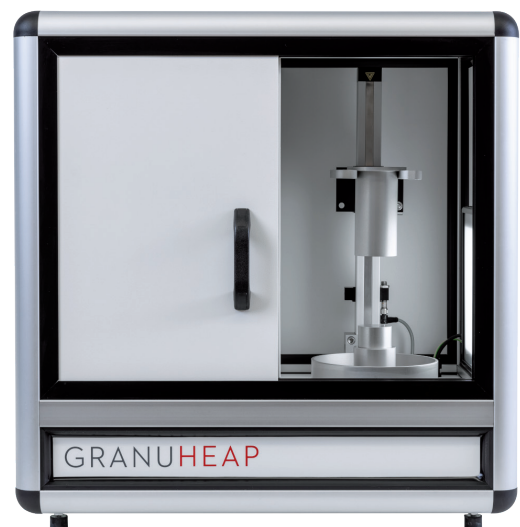
Figure 4: GranuHeap – an automated AOR measurement device.
