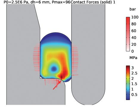
Figure 4: Pressurisation of the assembled O-ring from Figure 3.
