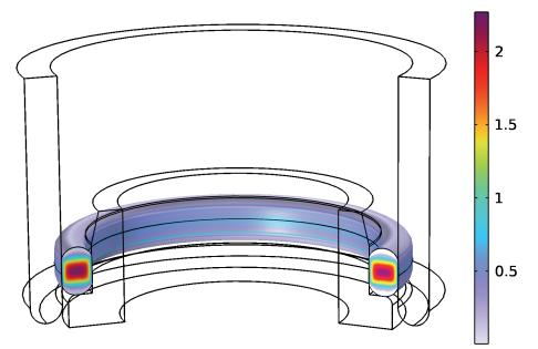
Figure 3: Hyperelastic FEA model of the assembly of two components and an LSR O-ring.
