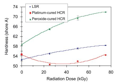
Figure 1: Effect of gamma radiation on durometer hardness of silicone rubbers.<sup>7</sup>
