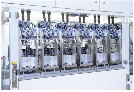
Figure 1: Process detail of an injector test system.
