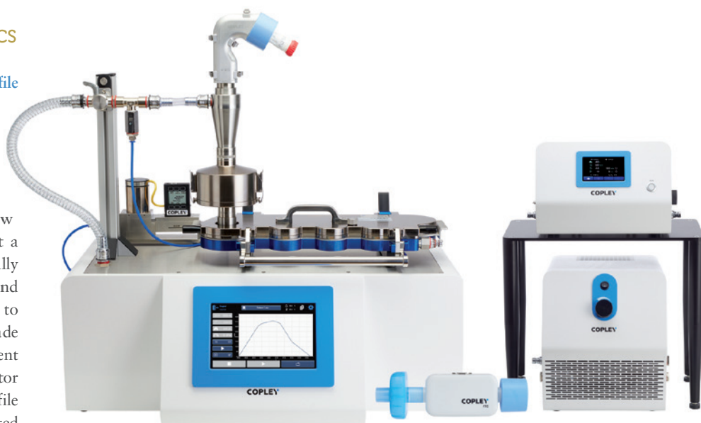
Figure 3: A test set-up for clinically representative DPI testing complete with breathing simulator, mixing inlet and AIT.
