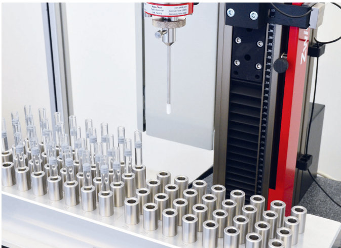
Figure 2: Serial testing with X-Y table for breakaway and glide force testing.
