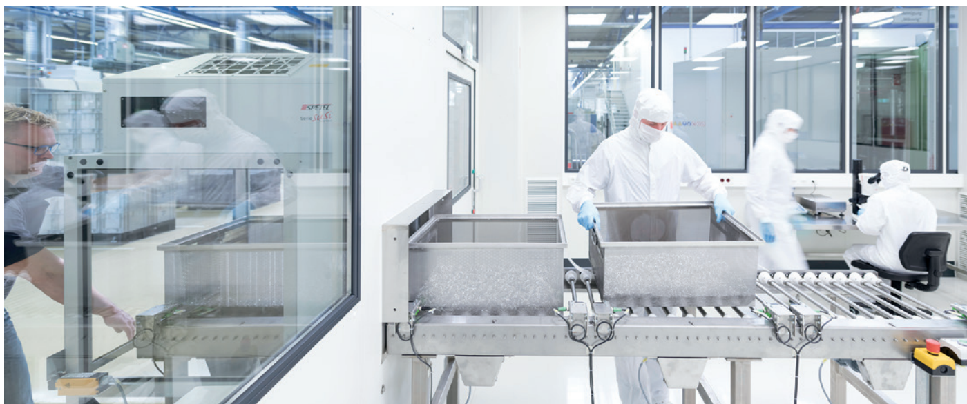
Figure 2: STÜKEN MEDICAL operates Class 7 cleanrooms in accordance with DIN EN ISO 14644 and EU GMP Class C guidelines.
