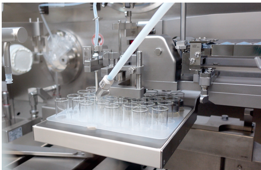
Figure 1: Grand River Aseptic Manufacturing cartridge filling for custom drug delivery innovations.
