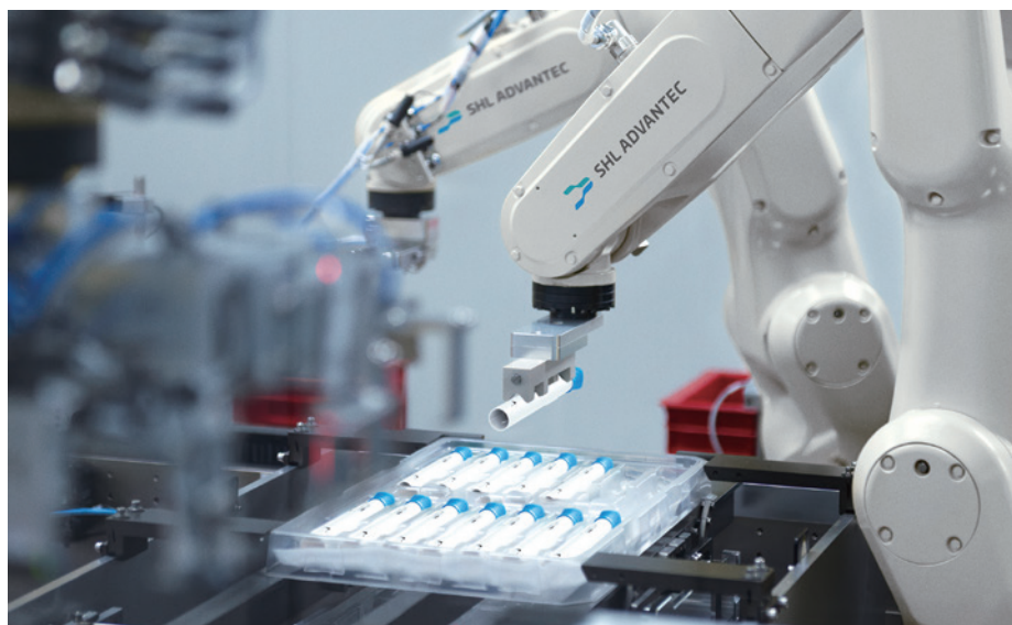
Figure 3: The SMART assembly machine uses an array of robotic arms that are programmed to migrate device components from feeding systems to moving shuttles.
