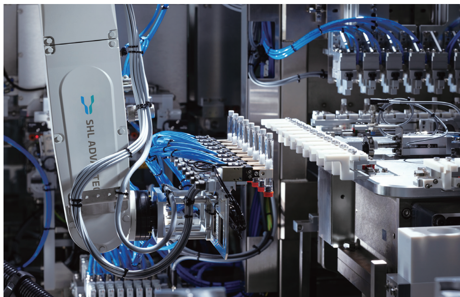
Figure 4: Fully modular final assembly machine with a fully automated primary container loader compatible with both tubs and trays.
