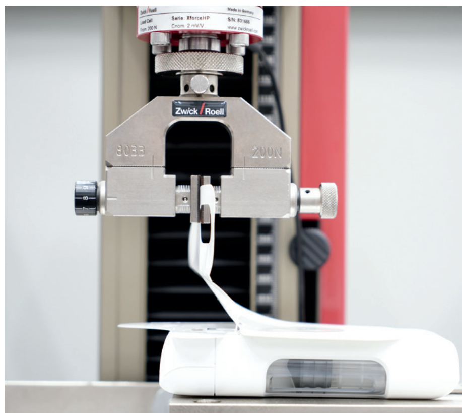
Figure 2: Peel forces for the film are determined in the peel test.
