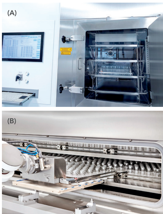
Figure 4: Scale-up – (A) from lab lyophiliser for small-scale studies to (B) automated, commercially operated lyophiliser.
