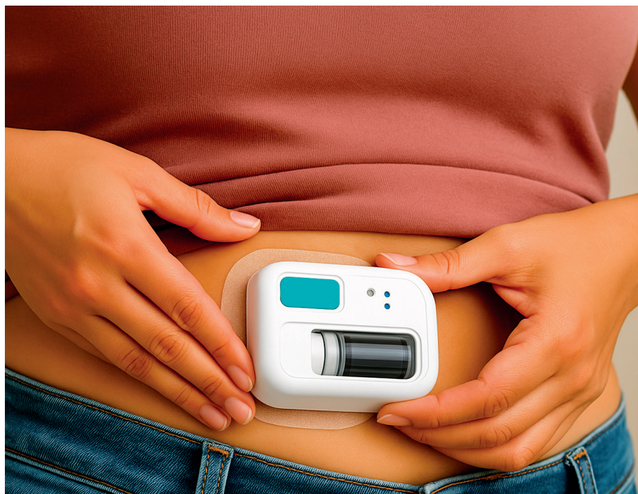
Figure 2: Wearable technologies are becoming the established solution for the delivery of high-dose (large-volume or high-viscosity) formulations.
