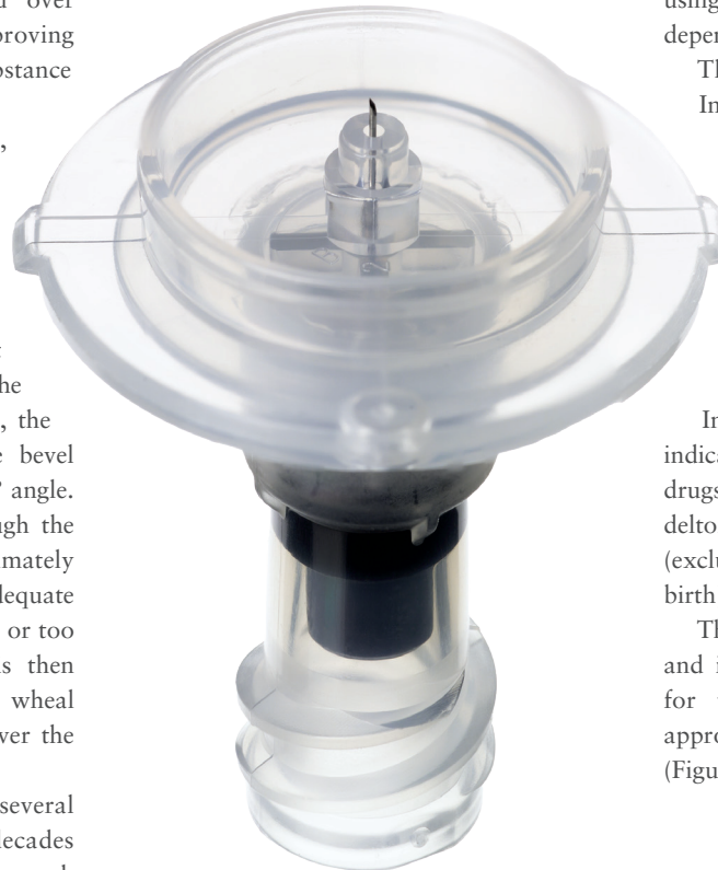
Figure 1: The needle-end of the Terumo Immucise™ ID injection system, illustrating the outer diameter of 0.2 mm (33G) and length of 1.15 mm, which is designed to be retained in the dermal layer during delivery. 2
