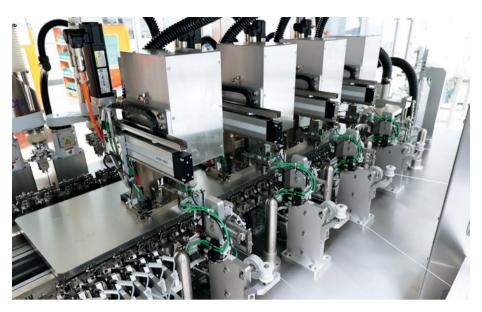
Figure 5: Servo-electric PnP.
