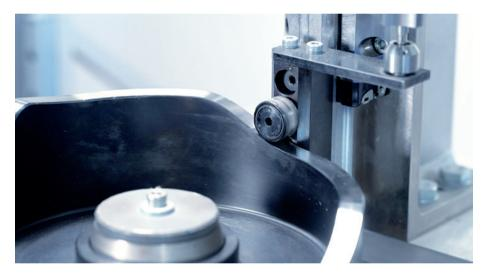
Figure 6: Detail of a cam drive.
