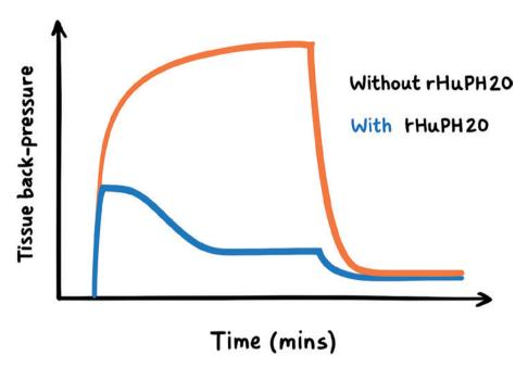
Figure 3: The effect of hyaluronidase adjuvant on the tissue back-pressure experienced during a 10 mL, 7 cP injection over several minutes. Note that the effect becomes apparent after a certain timescale during delivery and that a plateau is reached during the delivery. Reproduced from Pepin *et al* (2023).
