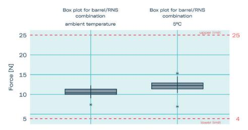
Figure 3: Box plot showing RNS pull-off force with optimised cone/RNS interface, ambient temperature versus cold storage 5°C (worst case).
