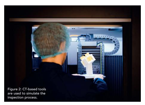
These tools support detailed analysis of geometry, manufacturing feasibility and part-to-part fit before physical tools are created. Simulations also enable early identification of potential risks, such as sink marks, air entrapment or misalignment. The resulting metrology plans are then directly applicable when real parts are produced, saving time and reducing trial iterations.
