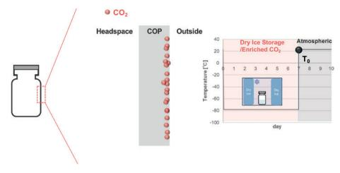
Figure 8: Schematic illustration of  ${\rm CO_2}$  dissolution in COP vials immediately after removal from dry ice.
