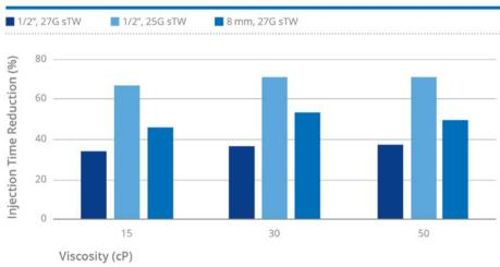
Figure 4: Injection time reduction relative to 27G TW 1/2". Note: For the 27G sTW categories at 50 cP, the values were derived from empirical measurements obtained in previous experimental studies.
