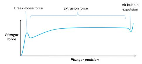
Figure 1: The force-distance chart for a BLEF test.
