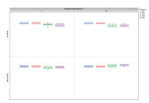
Figure 2: The gliding force (GF) for water-filled 5.5 mL syringes was tested on a universal test machine directly after filling (0 m) and after 1, 3 and 6 months of storage at 5°C and 25°C. The syringes were stoppered with a Datwyler NeoFlex<sup>™</sup> plunger.
