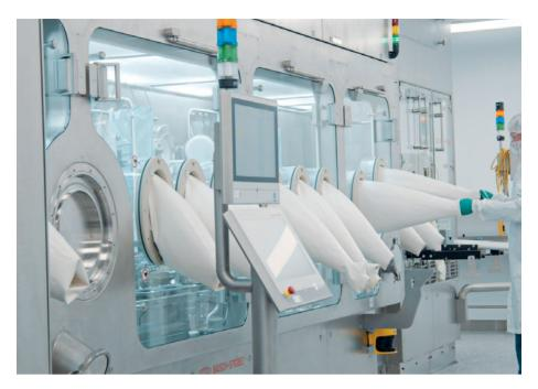
Figure 1: Specialist isolator technology may be required when filling highly sensitive biologics.
