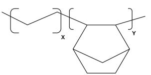
Figure 1: Chemical structure of cyclo-olefin copolymer.
