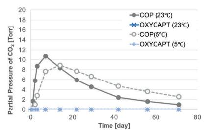
Figure 7: Changes in  ${\rm CO}_2$  partial pressure in vial headspaces after removal from insulated chamber.
