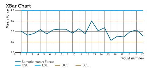
Figure 3: Control chart of force of 100 SPC measurements with sample size five. Point 12 has an average value higher than upper control limit, which triggers correction of the machine settings, and the average value of the next point reverts back to the target average.
