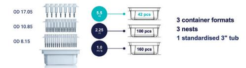
Figure 3: The syriQ BioPure® platform uses a standardised 3" tub for all three volumes of pre-sterilised, nested prefillable syringes, designed to facilitate automated fill-finish. The tub is sealed with a Tyvek® sheet and packaged in a double-bag configuration. OD: outer diameter of the glass barrel.
