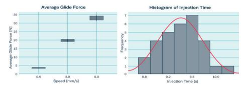
Figure 4: Liquid-dependent performance features: average glide force (1) and injection time (2) of a 2.25 mL Gx<sup>®</sup> Elite syringe 27 G thin wall, ID 0.28 mm, with PremiumCoat<sup>®</sup> plunger mounted in SHL Molly; tested with 15 cPs water-based solution.
