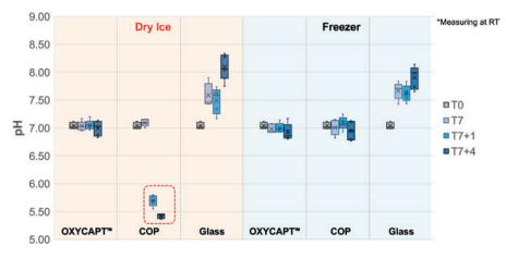
Figure 10: pH variation of distilled water after dry ice storage.
