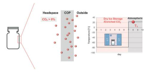
Figure 9: Schematic illustration of CO<sub>2</sub> diffusion through COP vials one day after removal.
