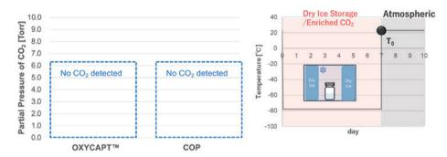
Figure 5: CO<sub>2</sub> measurements in vial headspace immediately after removal.
