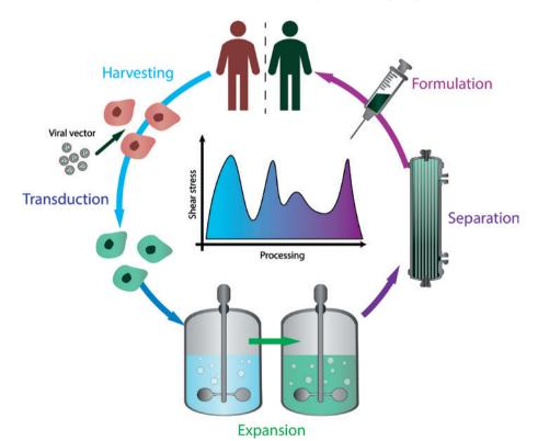
Figure 1: This schematic outlines some major workflow stages in CGT manufacture: harvest and transduction, expansion, separation and final formulation for patient delivery. When unmanaged, shear stress can fluctuate sharply across CGT manufacturing at any of these stages.
