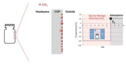
Figure 8: Schematic illustration of  ${\rm CO_2}$  dissolution in COP vials immediately after removal from dry ice.
